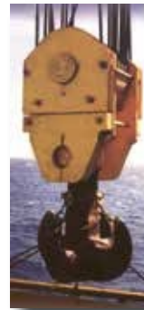
600 tonnes WLL Offshore Service Block. Quadruplex Hook
