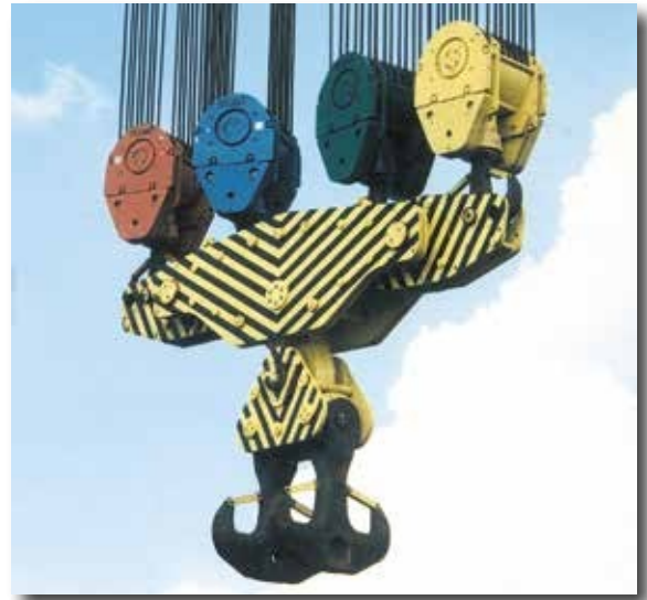
Mega Lift 3000 tonnes WLL Crane Ship Lifting System
