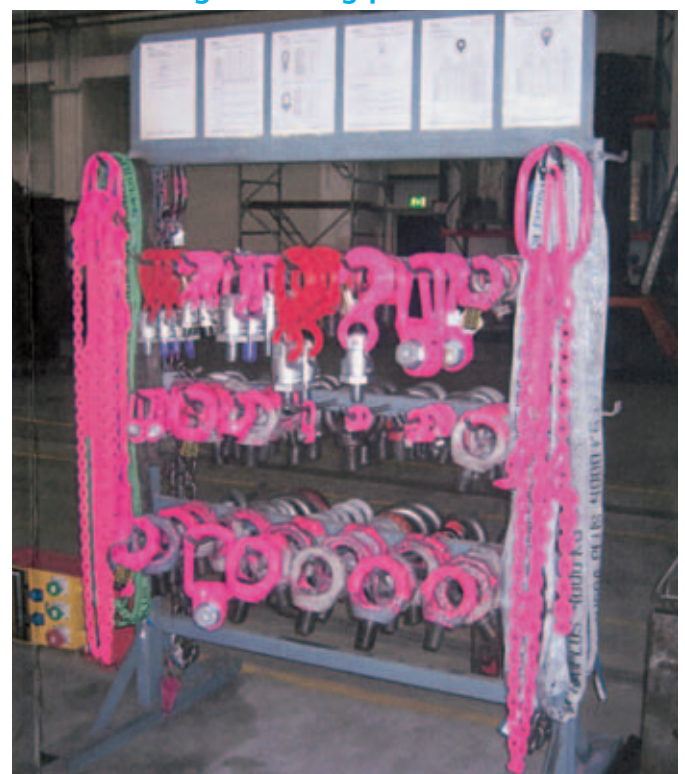
Correct storage of lifting points and sling chains BGR 500.
